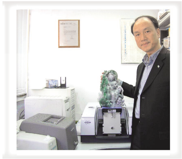
Large Jadeite carving being tested for infrared reflection spectrum.
